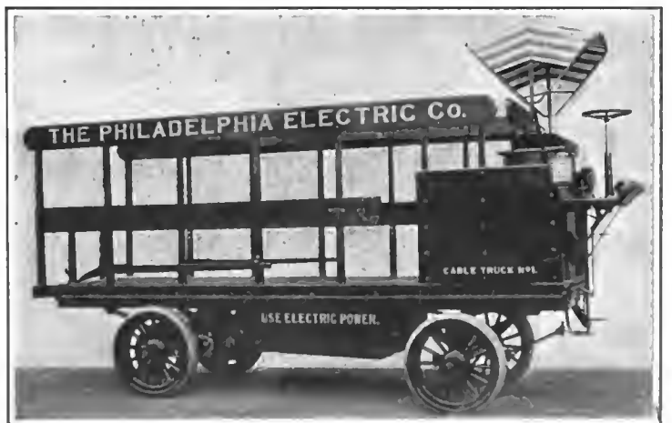
COLUMBIA ELECTRIC CABLE TRUCK WITH WINDLASS.
